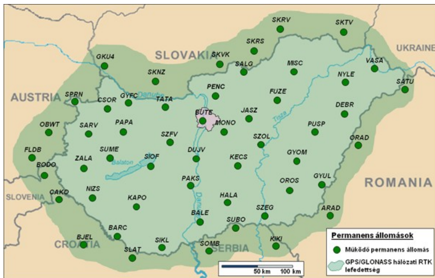
RTK networking coverage of Hungary towards the end 2009 ( www.gnssnet.hu )
